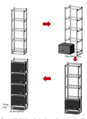
Figure 4-1: Battery Module Installation (A possible battery install procedure)
