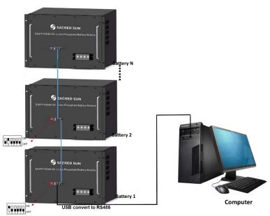
Figure 5-5: Communication Cable Connections among Multiple Batteries
