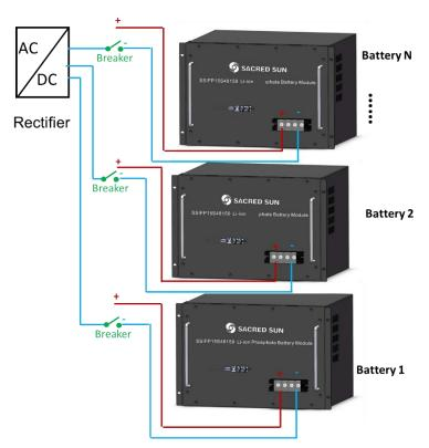
Figure 5-4: Multiple Batteries Connections
