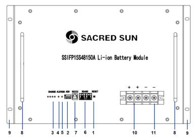
Figure 2-2: Front Panel Function Introduction
